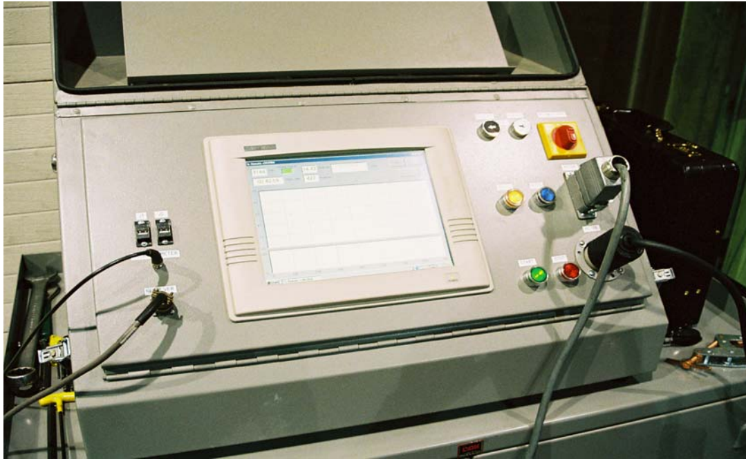
Figure 3: VSR-8000 Console. The console features an industrial grade, touch-screen PC which displays all pertinent vibration data, and includes several process controls. The pushbuttons (to the right of the PC screen) control vibrator start / stop, automatic/manual scanning, and vibrator RPM increase / decrease pushbuttons.
