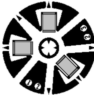
Figure 2.1.1: Strain Gage Arrangement for Measuring Residual Stress (Micro Measurements, 2004).
