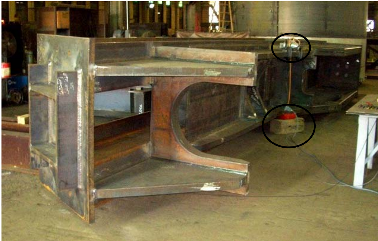
Figure 1: View from near one end of the 30-ton Ingot Stripper Frame. The Frame was isolated on 3 Isolation Load Cushions (1 is visible [circled], midway down the length of the Frame). Each Load Cushion was placed on a 10" X 10" wood block to achieve leveling and floor clearance (Frame is \approx 4" above the floor in the foreground.) The BL-8 VSR Vibrator, clamped to the Frame, can be seen directly above the Cushion (circled).
