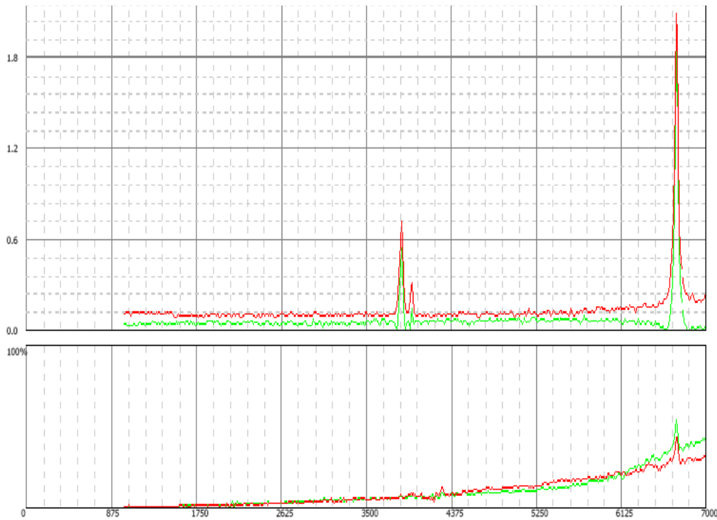
FIGURE 7. Treatment Chart: Treatment 1B. The red Post-Treatment Scan documents growth of 16% of the 6685 RPM peak. The previously treated, smaller peaks also grew, a common occurrence during the VSR Process. Treatment time was 26 minutes.
