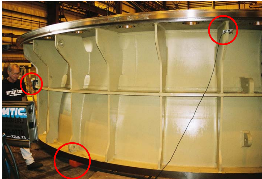
FIGURE 2. One of three orange Isolation Load Cushions can be seen in the left foreground (circled). The second Load Cushion (not visible) was placed under that area of the workpiece in the right foreground, 6' to the right of the visible cushion. The third Load Cushion was opposite the midpoint between these two, under the far side of the workpiece. The Accelerometer is clamped on the upper right of this image (circled). One of the Vibrator's clamps is visible to the right (circled) of the VOITH-SIEMENS employee.
