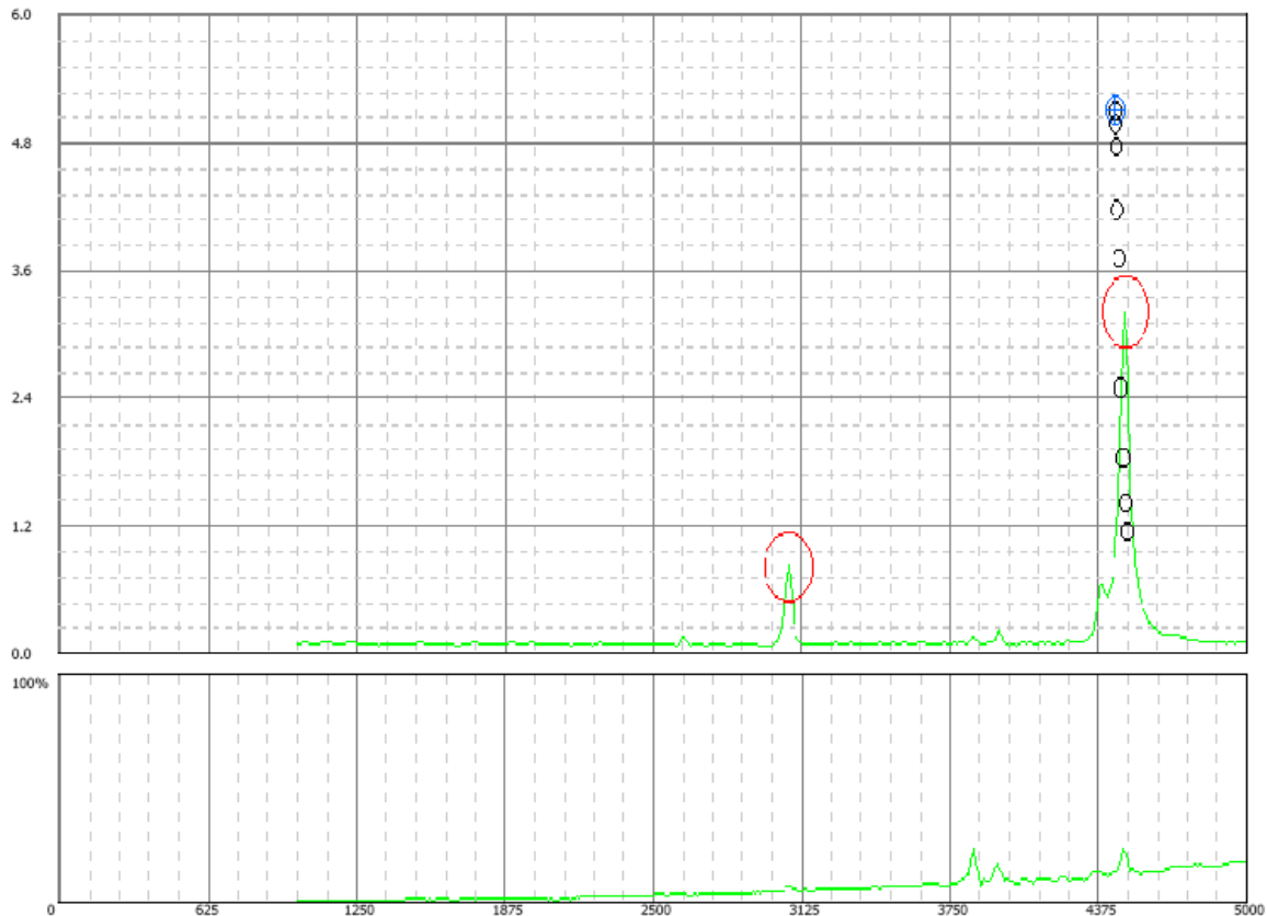
FIGURE 9. Pre-Treatment Scan: Treatment 2. The vibrator's AOR was vertical, the vibrator unbalance set at 40% (1.6 in-lbs), and Accelerometer oriented to be sensitive to radial amplitudes. The short peak at 3060 RPM did not grow. The extremely narrow peak at 4485 RPM grew 37% during Treatment, but this growth was difficult to distinguish when comparing Pre-Scan and Post-Scan, due to the peak's very narrow shape, and the large inertia of the workpiece. Peak growth can be clearly seen, however, when using the system's AutoTreat software, by observing the Progress Dot patterns. The interval between Progress Dots is selectable, at intervals of 15, 30, 60 and 180 second spacing. On the Pre-Treatment Scan, shown above, a 60 second Progress Dot spacing was used. The blue, real-time cursor at the top of the peak indicates that this image was saved at the end of this VSR Treatment.
