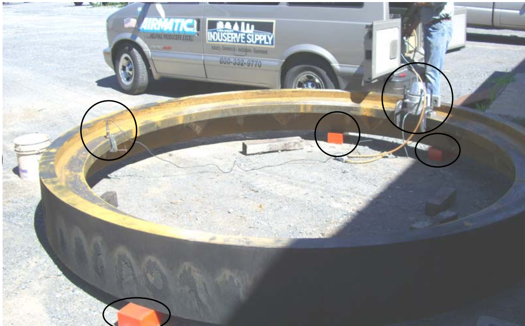
Figure 1: 3 Isolation Load Cushions (circled) support the 5-ton welded Ring, two are near the Vibrator on right, one is opposite in left foreground, positioning that minimizes workpiece damping. Vibrator (circled upper-right, inside) was securely clamped with orientation in the radial AOR during this 2 nd Treatment. Accelerometer (circled on left, inside), is positioned in the area of maximum amplitude.
