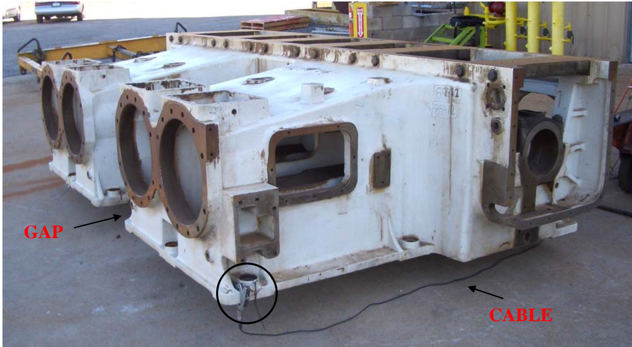
Figure 2: "Gap" side on left is \approx 20 ". A Load Cushion was placed on each side of the gap (not visible), about 12" from the outer edge of the Frame. The Accelerometer can be seen in the foreground (circled), with its connecting cable leading to the VSR-8000 Console.
