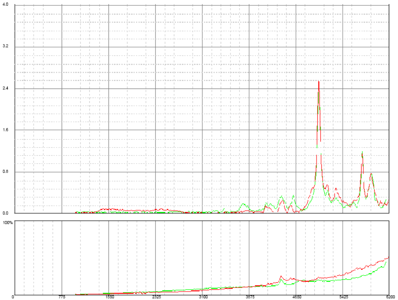
Figure 5: Workpiece 1, Treatment 2. Relocation and re-orientation of the Accelerometer enabled high RPM peaks to be easily detected. However, little peak growth or shift took place, as evidenced by the similar Pre- and Post-Treatment Scans.
