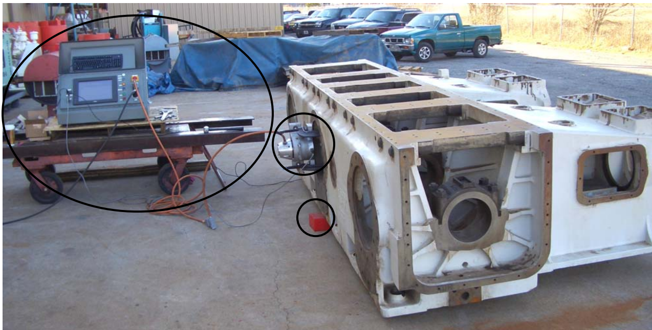
Figure 1: Compressor Frame setup for VSR Treatment. One Isolation Load Cushion (circled) is centered along continuous (non-gap) side of frame. The Vibrator (circled) was mounted above it. MX-8000 Console with touch-screen PC and USB keyboard visible on the left (circled).
