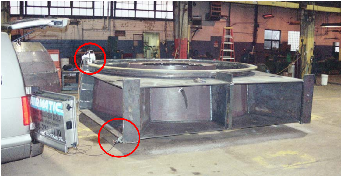
Figure 3: VSR SETUP. Weldment lowered to be aligned with horizontal plane (to minimize damping), and placed on 3 Isolation Load Cushions (not visible) located immediately underneath the flange ID. The Vibrator (circled) is attached to the top flange. Accelerometer (circled) is clamped to base of workpiece, and oriented to be most sensitive to vertical deflection of workpiece during vibration.
