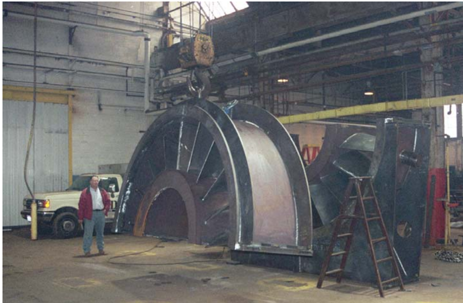
Figure 10: Fan Housing's upper half was lifted from the lower half during separation.
