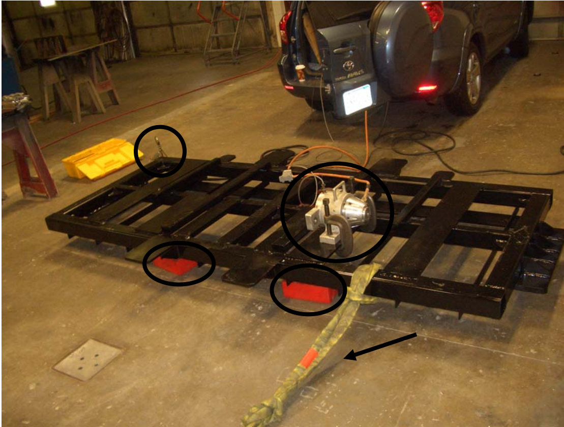
Figure 1: 1/2 ton Frame, setup for VSR Treatment. The Frame was set on 3 Isolation Load Cushions. Two are visible in the photo foreground (circled), and the third is obscured by the Vibrator (circled), on the far side, centered. The Vibrator was clamped on a stiff cross-member, and oriented so that its Axis of Rotation was parallel (AOR-P) to the length of the Frame. An Accelerometer was clamped on the far left corner (circled), oriented so as to be most sensitive to vertical deflections. Since the Frame was light, it started to walk off the Cushions during Treatment, so it was then tethered to the floor by the lifting strap in the foreground (arrow).
