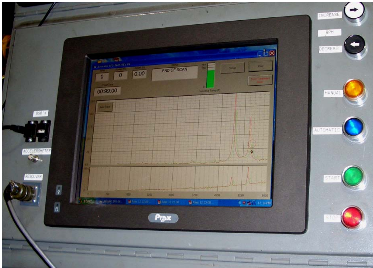
Figure 5: Close-up of 15" (38 cm) touchscreen PC, displaying the completed VSR Treatment Chart shown in Figure 4. To save the data, the operator prints the screen as an Adobe / pdf document. Other display data (not recorded on charts) but visible on the VSR-8000 System Main Operating Screen include (from left to right, starting at the top): Vibrator RPM, Vibrator input power (watts), Workpiece acceleration ( XX.XX , gs ), and an electronic bargraph / thermometer showing the Vibrator motor's winding temperature. Due to a combination of the rugged vibrator design and electronic motor protection, VSR Vibrators (along with VSR Systems in general) are very reliable.
